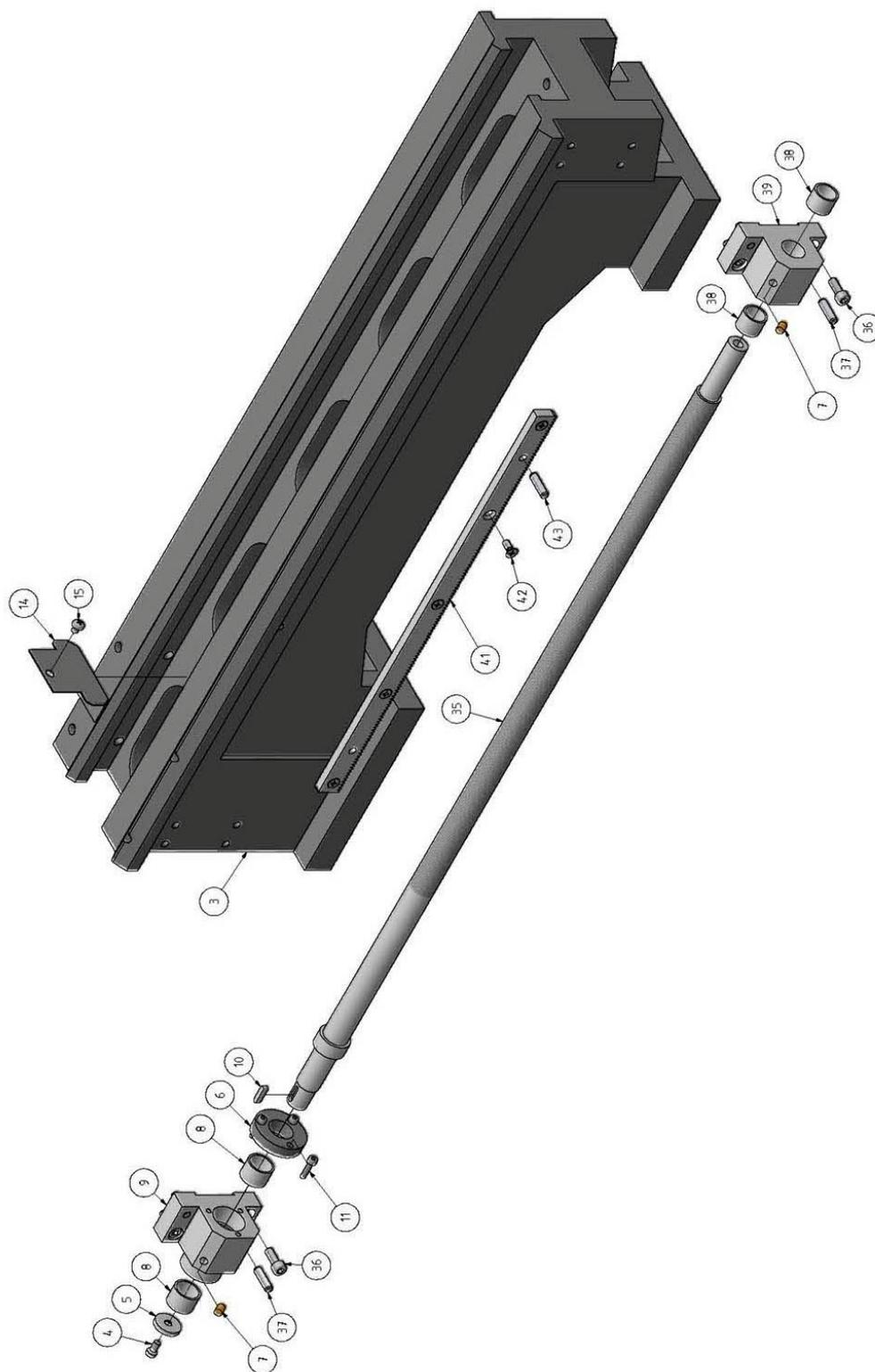
Abb.8-9: Maschinenbett - Lathe bed
