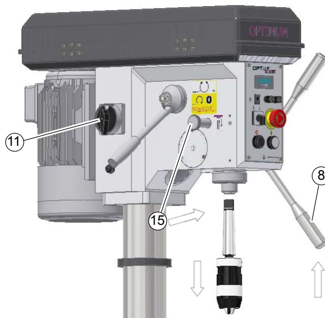
Img.4-7: Disassembly with integrated drill drift
