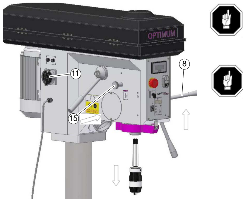
Img. 4-11: Disassembly with integrated drill drift
