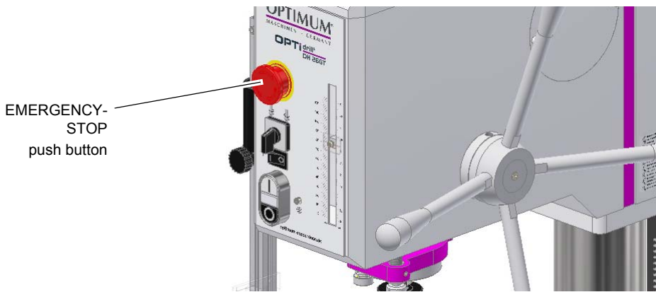
Img.1-2: Emergency stop
