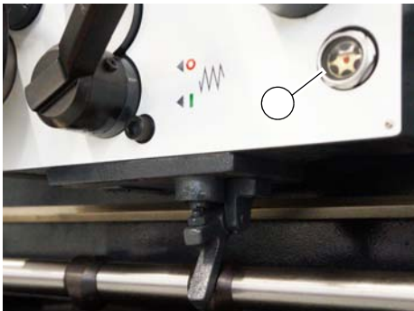
Oil sight glass apron
