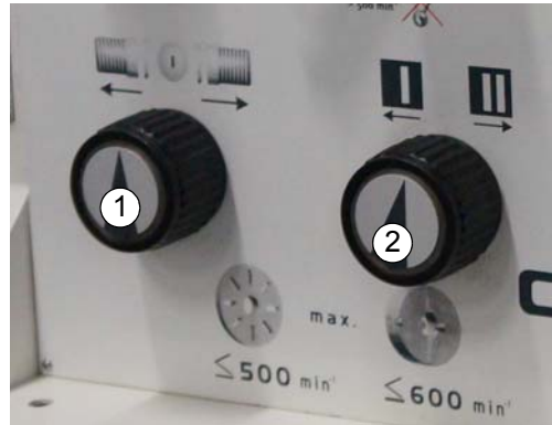
Feed direction (1) Infeed speed (2)
