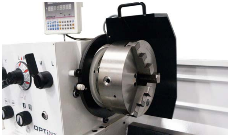
Img.1-4: Lathe chuck protection
