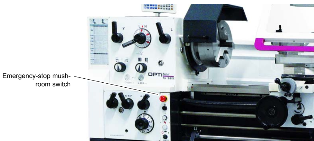
Img. 1-2: emergency-stop mushroom switch
