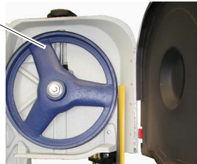
Img.3-6: Belt guide pulley
