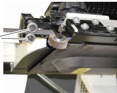
Img.3-7: Blade guide bearings
