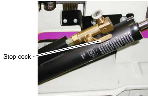
Img. 4-1: Hydraulic feed
